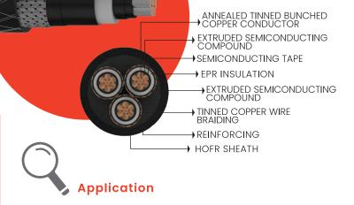
POLYCAB MV CU IS 9968-2 of voltage grade 6.35/11 KV (E) or 6.6/6.6(UE) KV, annealed tinned copper conductor, conductor screening, EPR insulated, insulation screening, HOFR sheathed single & multi core cable is suitable to use in mines, steel mills, wind power mills, ships, textile and construction machines and turbines.
